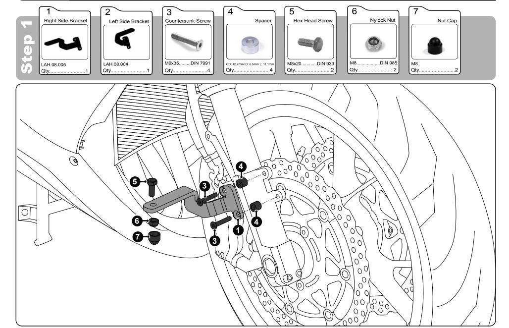
**Step One:** Remove the front fender to expose the mounting points illustrated above. Use the bolts (#3) and spacers (#4) to mount the left and ride side brackets (#1 & #2) to the motorcycle use the OEM fender bracket as the backing plate. Use the remaining hardware, bolts (#5), Nuts (#6) and nut caps (#7) to mount the light pods to the brackets. Reinstall the front fender to the motorcycle.
